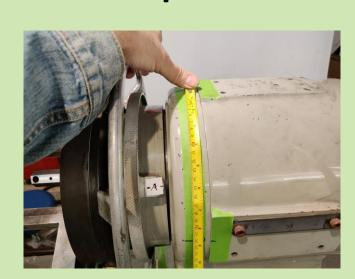
Step 6 Using the tape measure and table results lay out 10 degree marks 0-90
