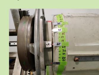
Step 9 This protractor can also be made using the absolute zero feature on a digital protractor held to the side of a chuck jaw and one of the set screw locations. Avoid buying a digital version that costs less than ~\$150. They can be unstable and inaccurate.
