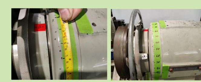
Step 8 Optional: Add sheet metal pointers to important angles for easier viewing
