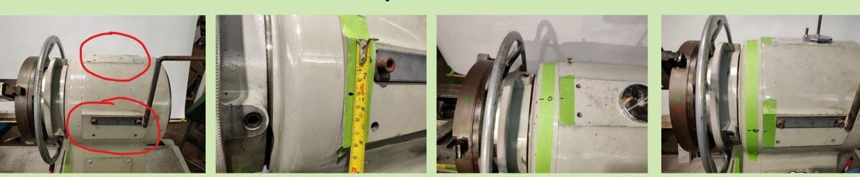
Step 3 Set an A at the front 90 location. Mark the back side location with the same color and "B" Repeat with all 3 colors
