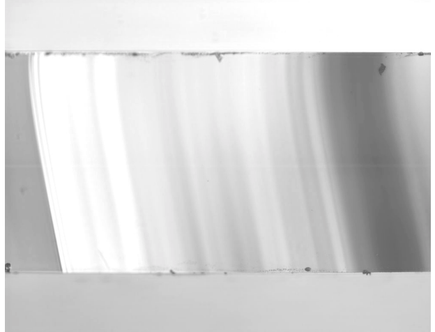
Fig. 9. Wallner lines on fracture surface Thermal stress is one stress that can generate this shape of Wallner lines. the crack runs right to left.
